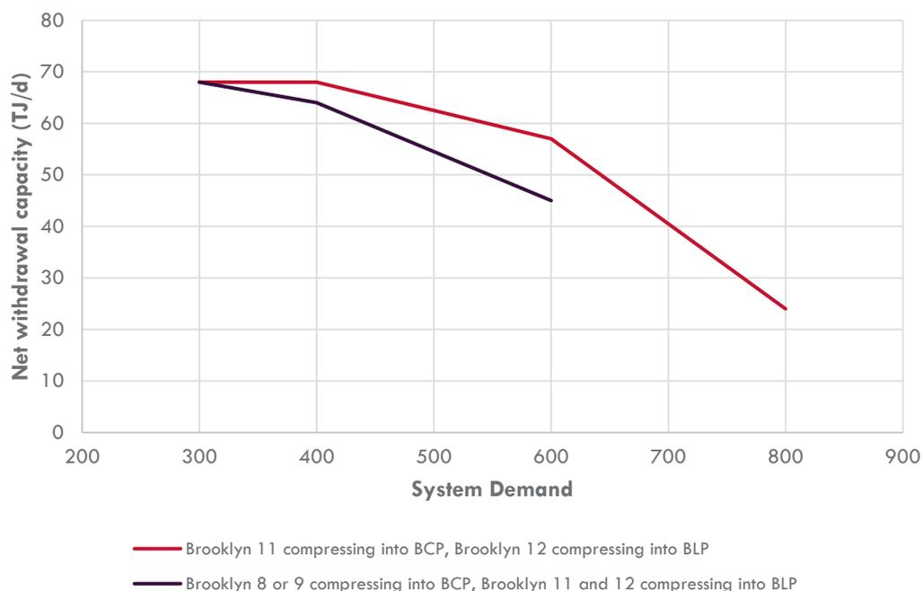
The impact of Laverton North PS operation on the SWP withdrawal capacity will vary between no impact when the generator is off, as shown in Figure 19, through to the generator operating at full rate, shown in Figure 20, depending on the rate of operation and operating hours.
