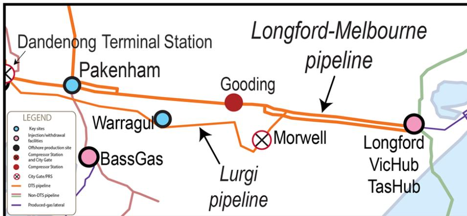
As set out in the 2017 VGPR, a pressure breach occurred at the Warragul CTM on 22 July 2014 when pressure dropped below the 1,400 kPa contractual minimum. Additional supply via the Lurgi backup regulators<sup>83</sup> located at the Dandenong Terminal Station has been used to maintain the Warragul supply pressure. This change was sufficient to support a peak instantaneous Warragul CTM flow of 10 kscm/h.
