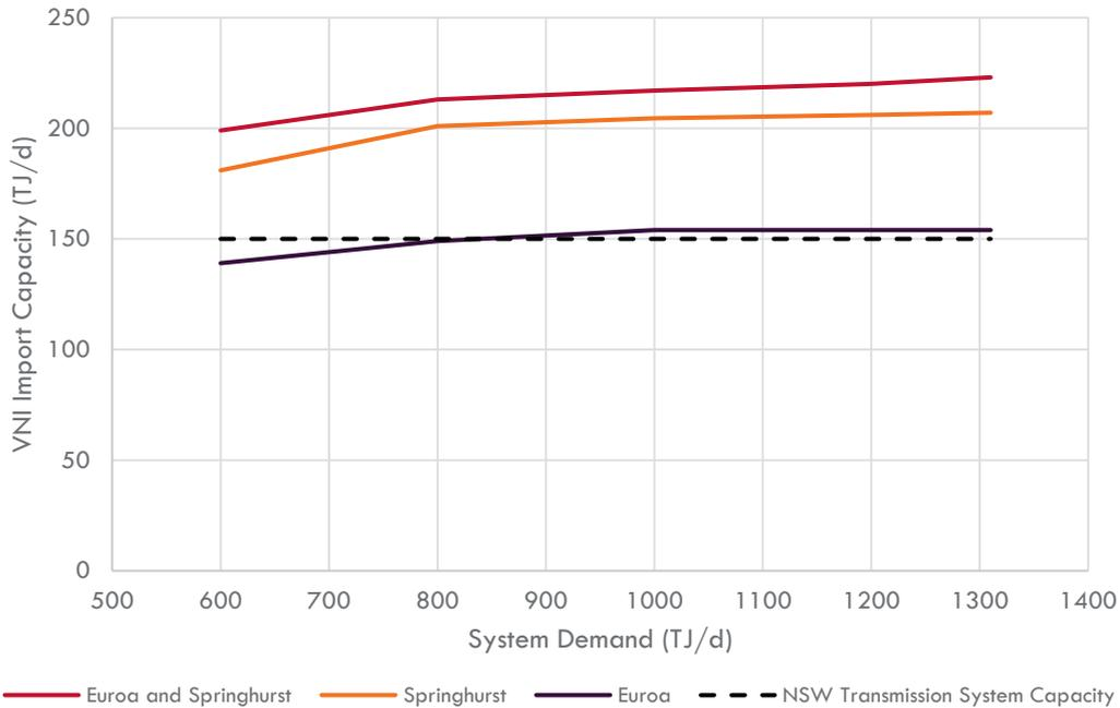
The Culcairn CS (which is part of the New South Wales transmission system) cannot currently compress gas in a southerly direction towards Victoria – it can only withdraw from the DTS. AEMO has observed that the Culcairn supply capacity into the DTS is reduced if the Uranquinty Power Station (which is supplied from the Young to Culcairn Pipeline) is operating, or during cold weather resulting in higher system demand on this pipeline.
