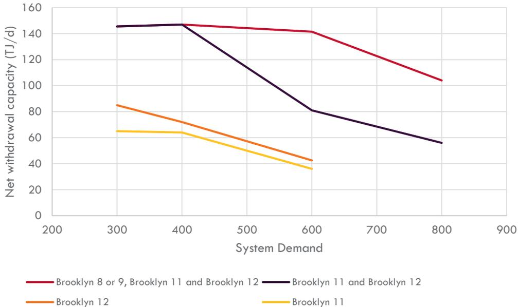
The maximum SWP withdrawal capacity of 147 TJ/d is achieved on a 400 TJ system demand day with Unit 11 and Unit 12 available. Before the augmentations were completed, the maximum SWP withdrawal capacity was 104 TJ/d.
