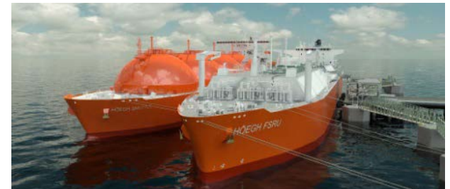
Floating Storage & Regasification Unit
