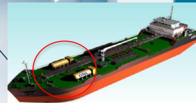
Virtual image of the barge with the two tanks added in the deck (the image shows 50m 3 tanks)
